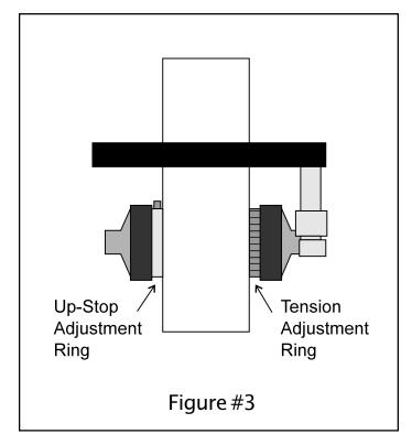
knobs. First loosen this ring to reset the mechanism by rotating the knob counter clockwise until you feel the tension release. Then tighten the knob by rotating it clockwise until it is "finger tight". The stage will now not raise above this location.
