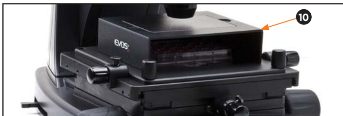
Light shield box ⑩ in place on stage
