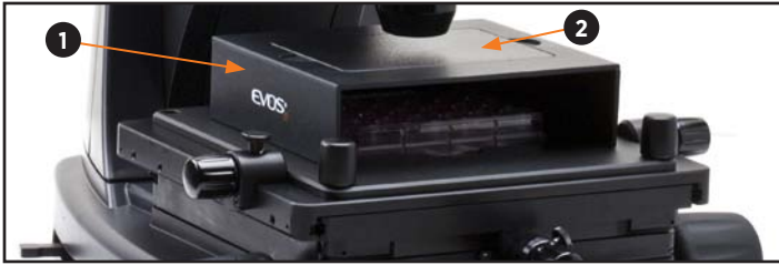
Light shield box ① in place on stage (cover ② shown in place)
