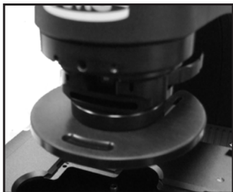
Condenser shield, removable
