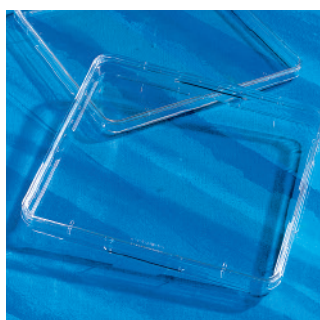
Figure 4. The Corning 245 mm square dish offers 500 cm 2 growth area.
