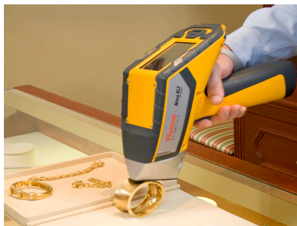
Jewelry analysis using a Thermo Scientific Niton XL2 analyzer.
