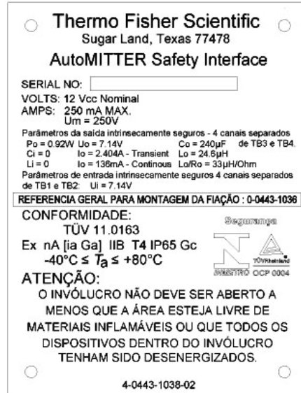
Figure 6–5. Certificate marking for Brazilian installations
