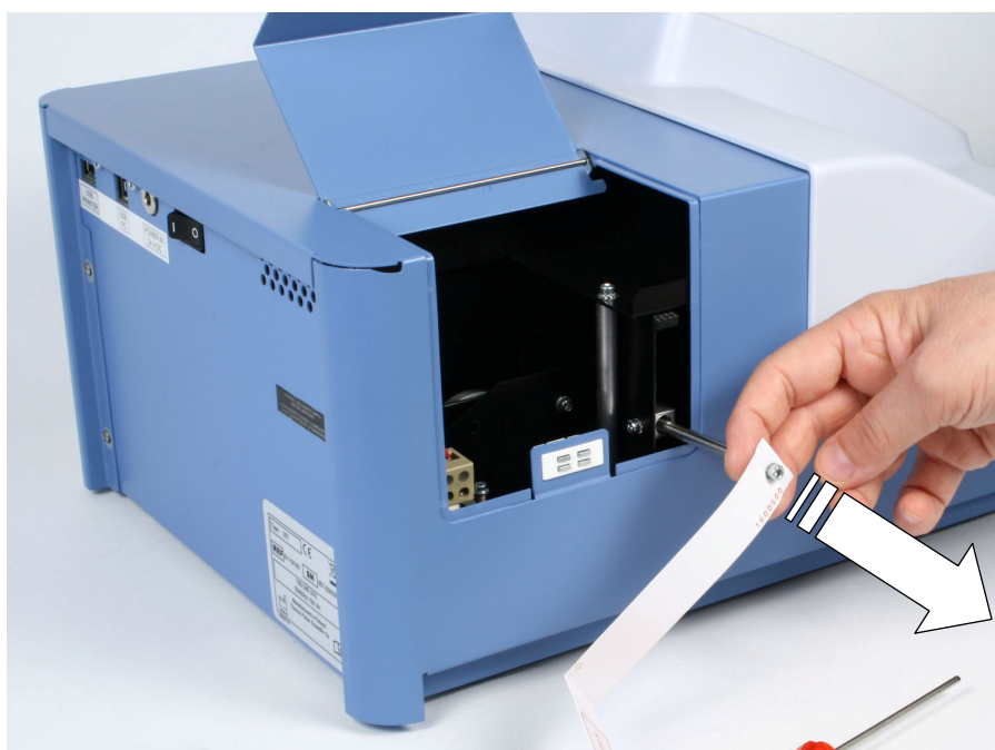
Figure 2–4. Pulling the transport lock out
