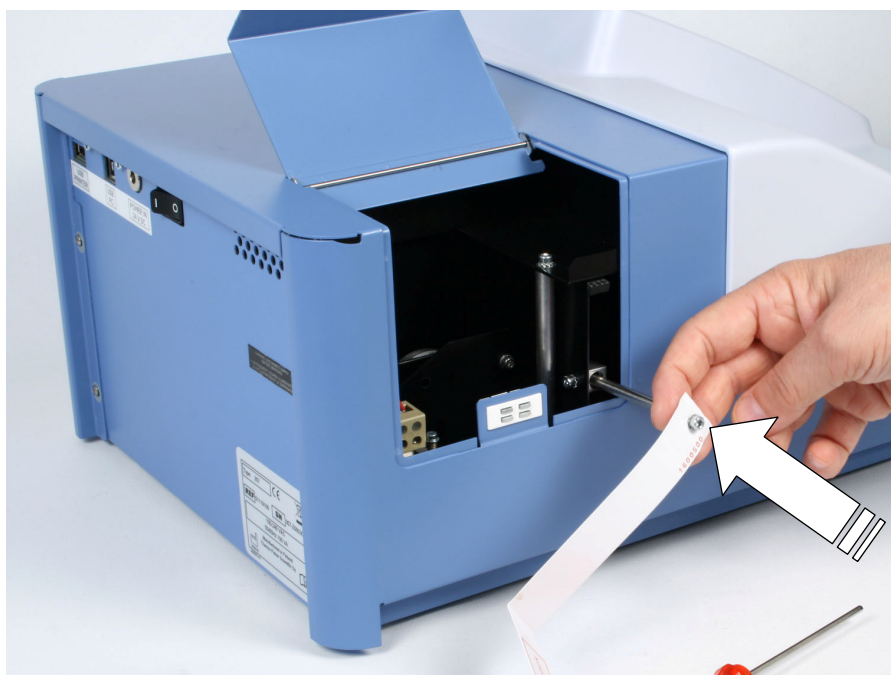
Figure 13–26. Refitting the transport lock bar into the measurement head
