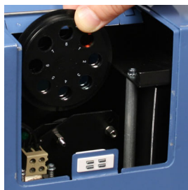
Figure 2–7. Placing the Multiskan FC filter wheel into the filter wheel slot
