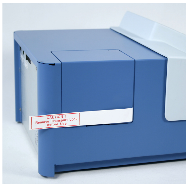
Figure 2–2. Transport lock (inside the instrument) and transport lock tag
