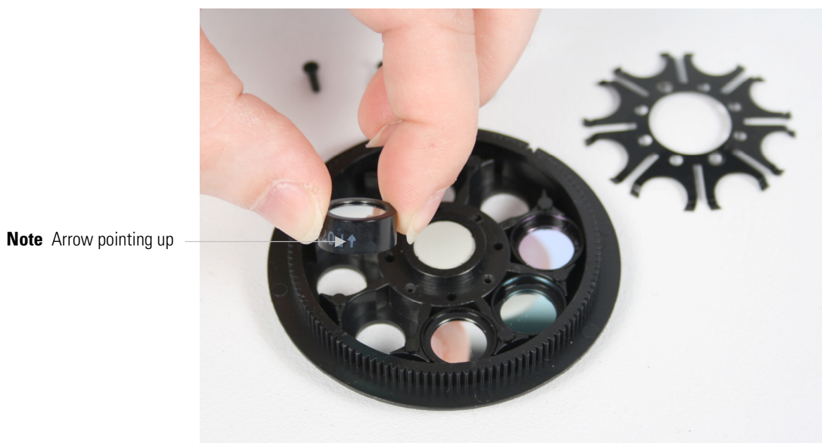
Figure 13-23. Inserting a filter into the next free position in the filter wheel
