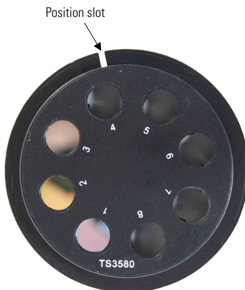
Figure 2–6. Multiskan FC filter wheel
