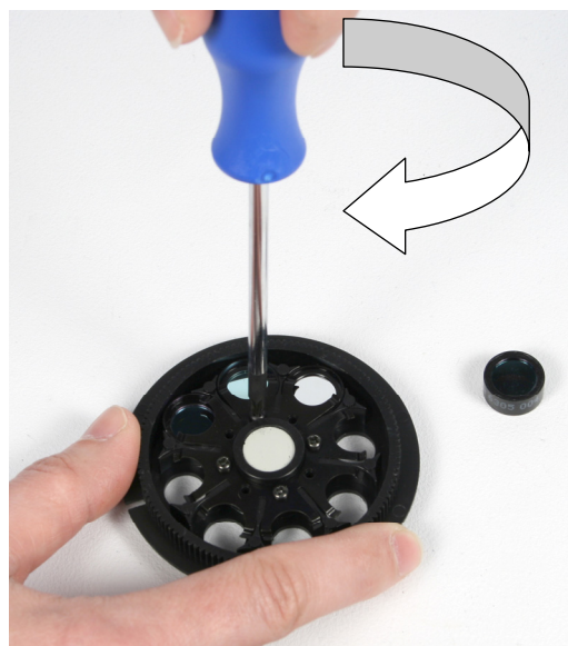
Figure 13-20. Removing the spring position holding screws
